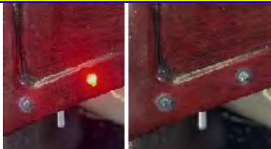
View of Toggle under dashboard and LED bulbs
